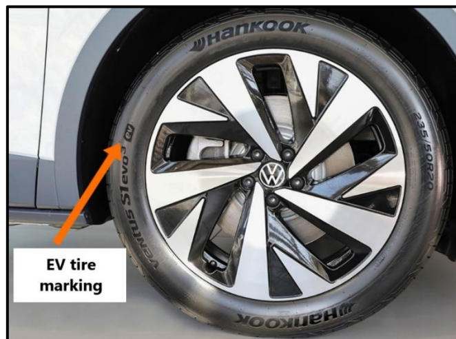
Figure 7. Electric vehicle (EV) tire marking [14].
