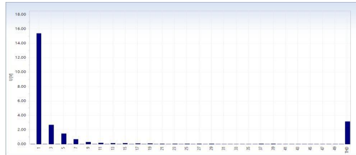
Fig.5: Measured voltage harmonic spectrum at PCC
