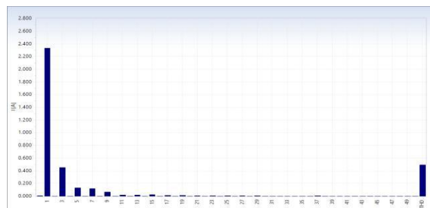
Fig.3: Measured current harmonic spectrum at PCC.
