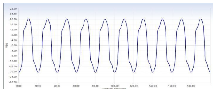
Fig.4: Measured voltage waveform at PCC.
