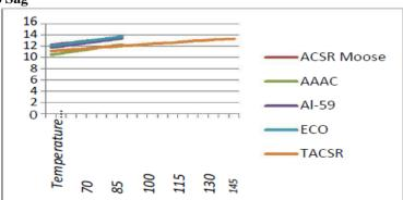
Thus Temperature VS Sag i.e. the line to ground clearance capacity of various conductors are compared.
