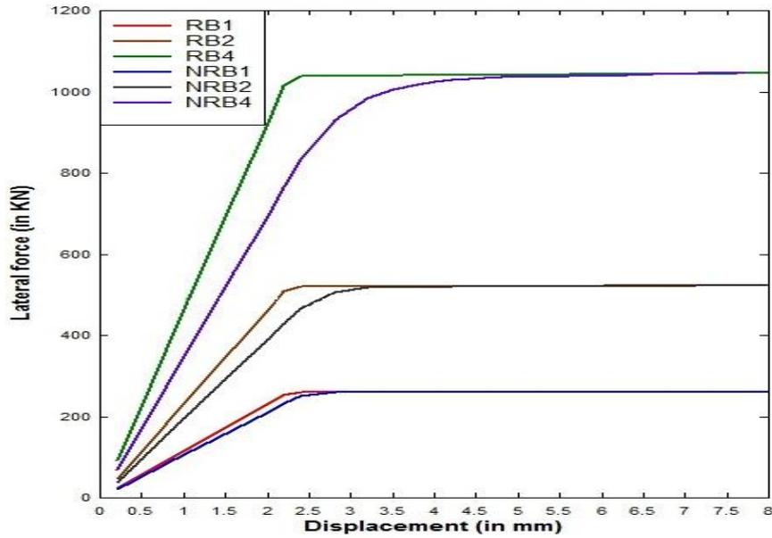
Fig. 6: Load displacement curves for RB1, RB2, RB4 and NRB1, NRB2, NRB4.
