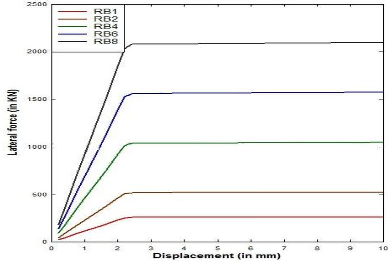
Fig. 5: Load displacement curves for RB1, RB2, RB4, RB6, and RB8.
