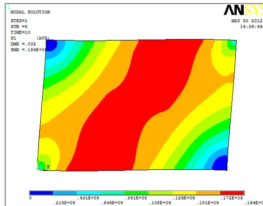
Fig. 10(b) Stress distribution for model NRB1
