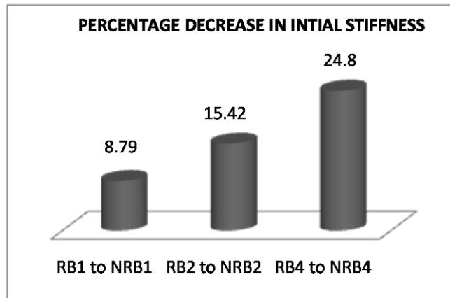
Fig. 9: Percentage decrease in the initial stiffness if frame members are made non-rigid.
