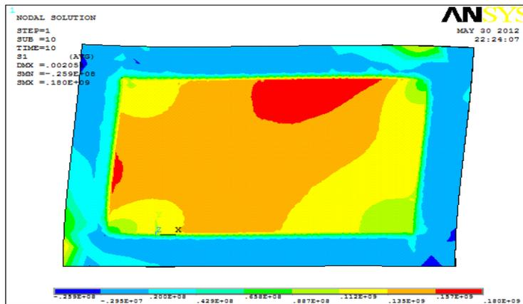
Fig. 10(c) Stress distribution for model M4 for a displacement of 2 mm
