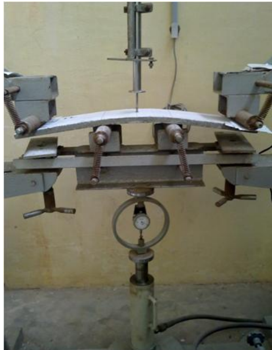
Fig. 5 Ductility of Ferrocement Slabs
