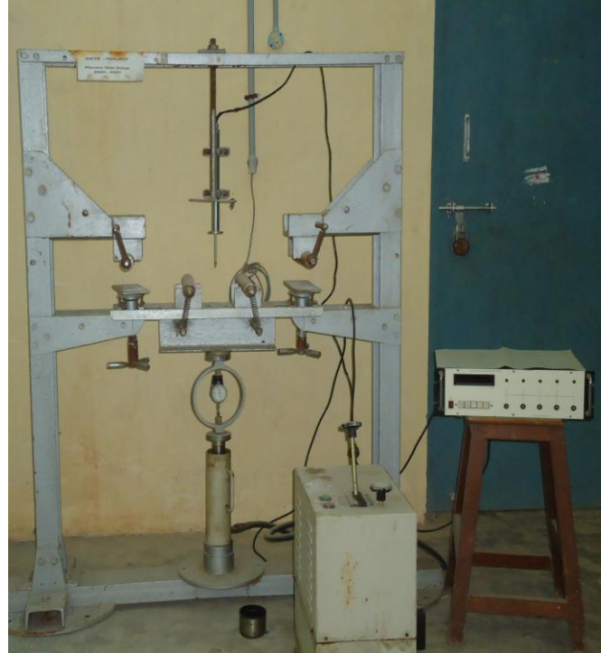
Fig. 2 Flexure Test Set-up
