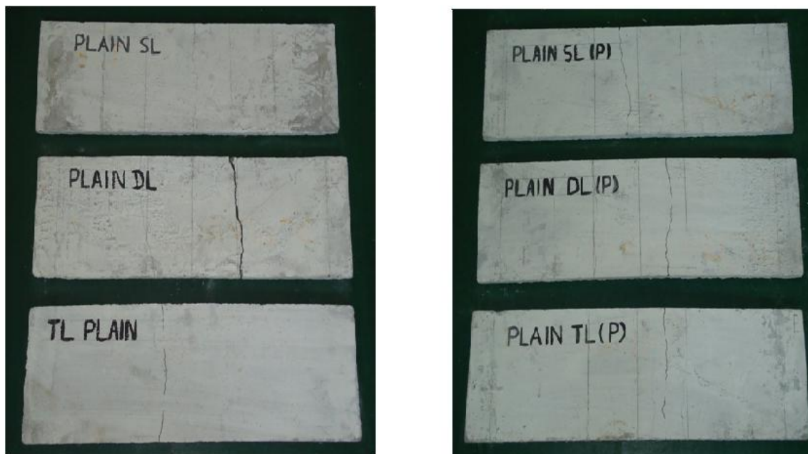
Fig. 8 Typical Crack-Pattern of Ferrocement Slabs cast with GI and PVC coated Weld Mesh, on ultimate failure loads
