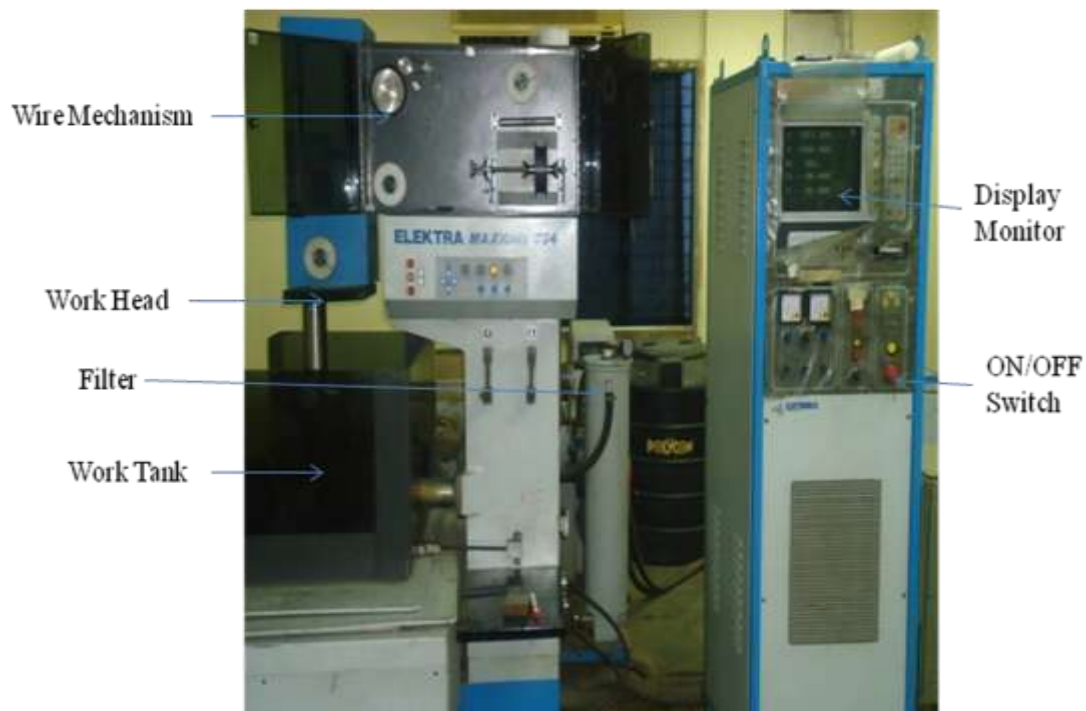
Figure 2: 'ELEKTRA MAXICUT 734', Electronica Machine Tool Ltd
