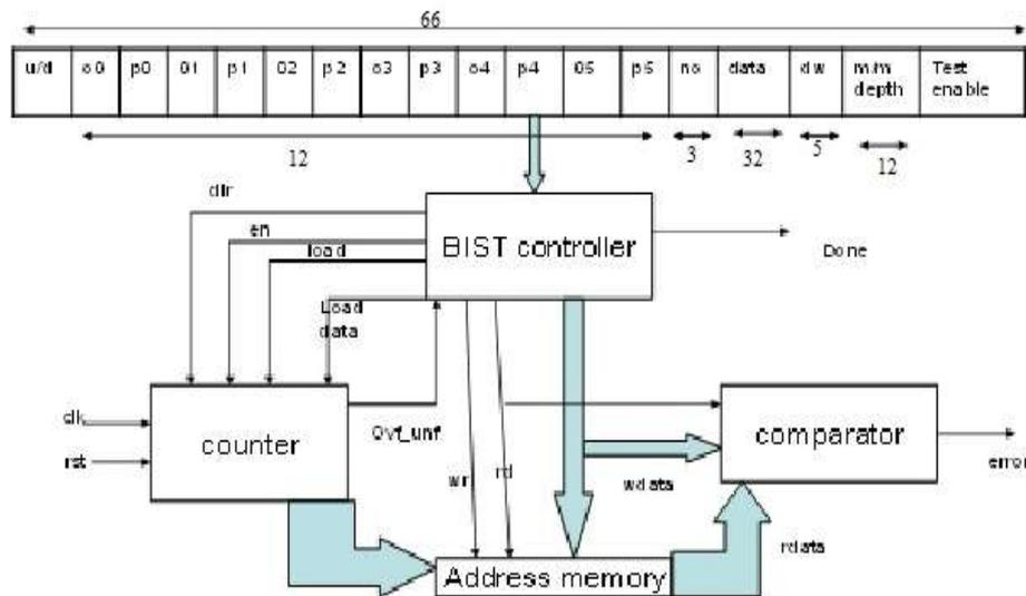
Figure 2: Proposed Architecture for Programming March C- Algorithm
