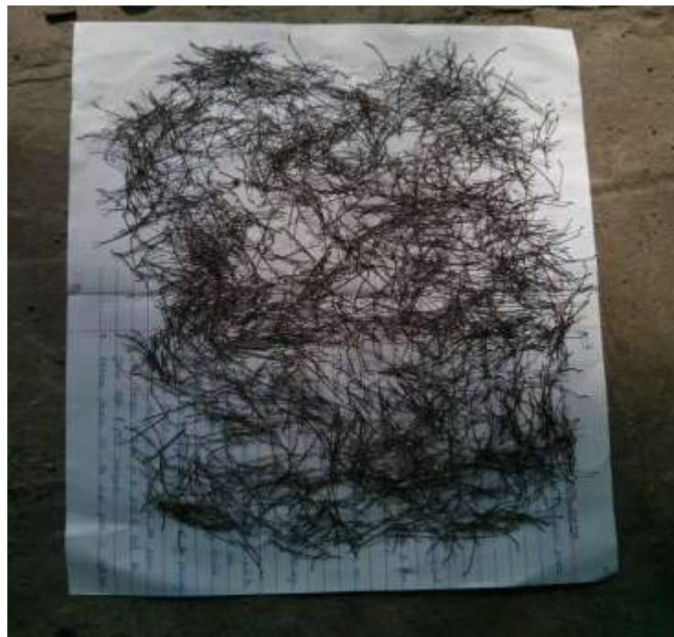
Fig: 4 Hooked End Steel Fibers used in study
