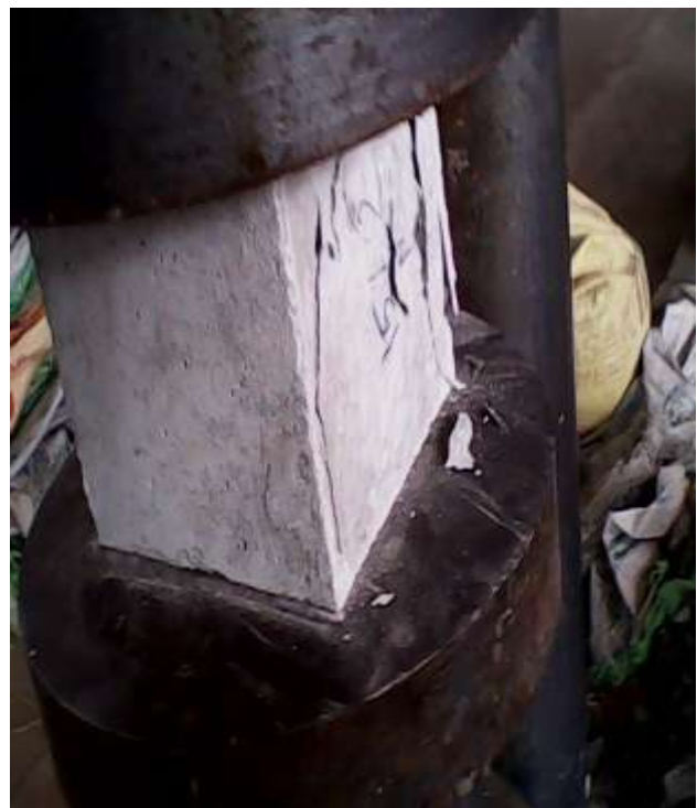
Fig.7 Cube failure after testing
