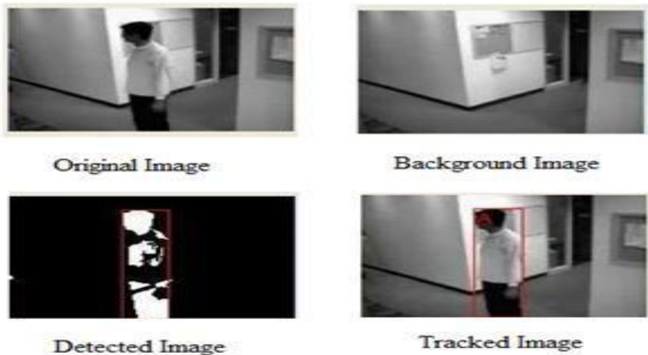
Fig.5: Each subfigure shows one camera at one of four time instants denoted by T. The track of one target, marked with a box. All targets are tracked using the Kalman-Consensus filtering approach, but are not marked for clarity. Tracked image at time T=2.2 sec.
