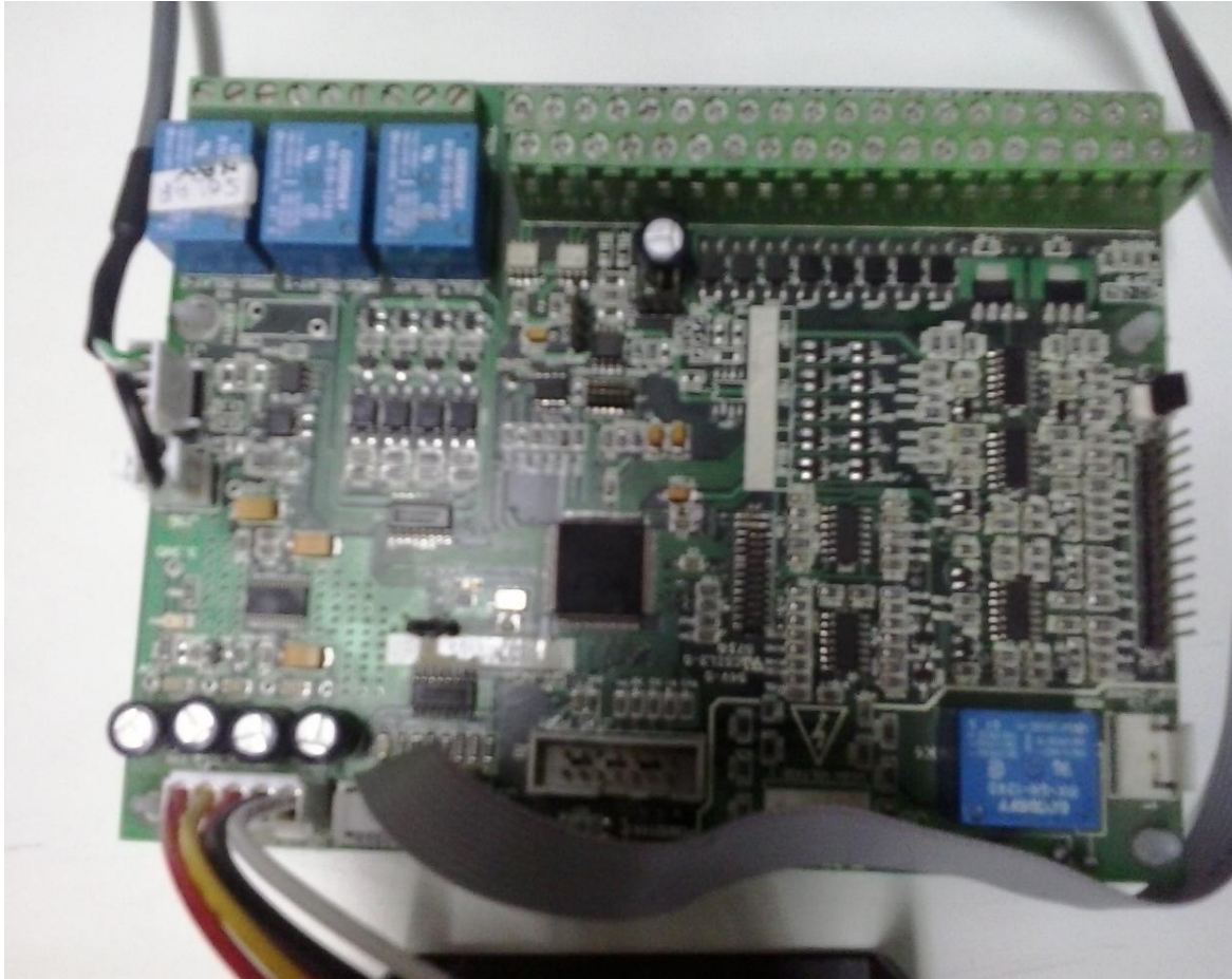
Fig. 2: PCA-2014 board based on TMS320F2811 DSP by Texas Instruments®
