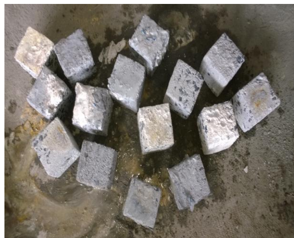
Fig.6 Cubes after curing in MgSO 4 solution
