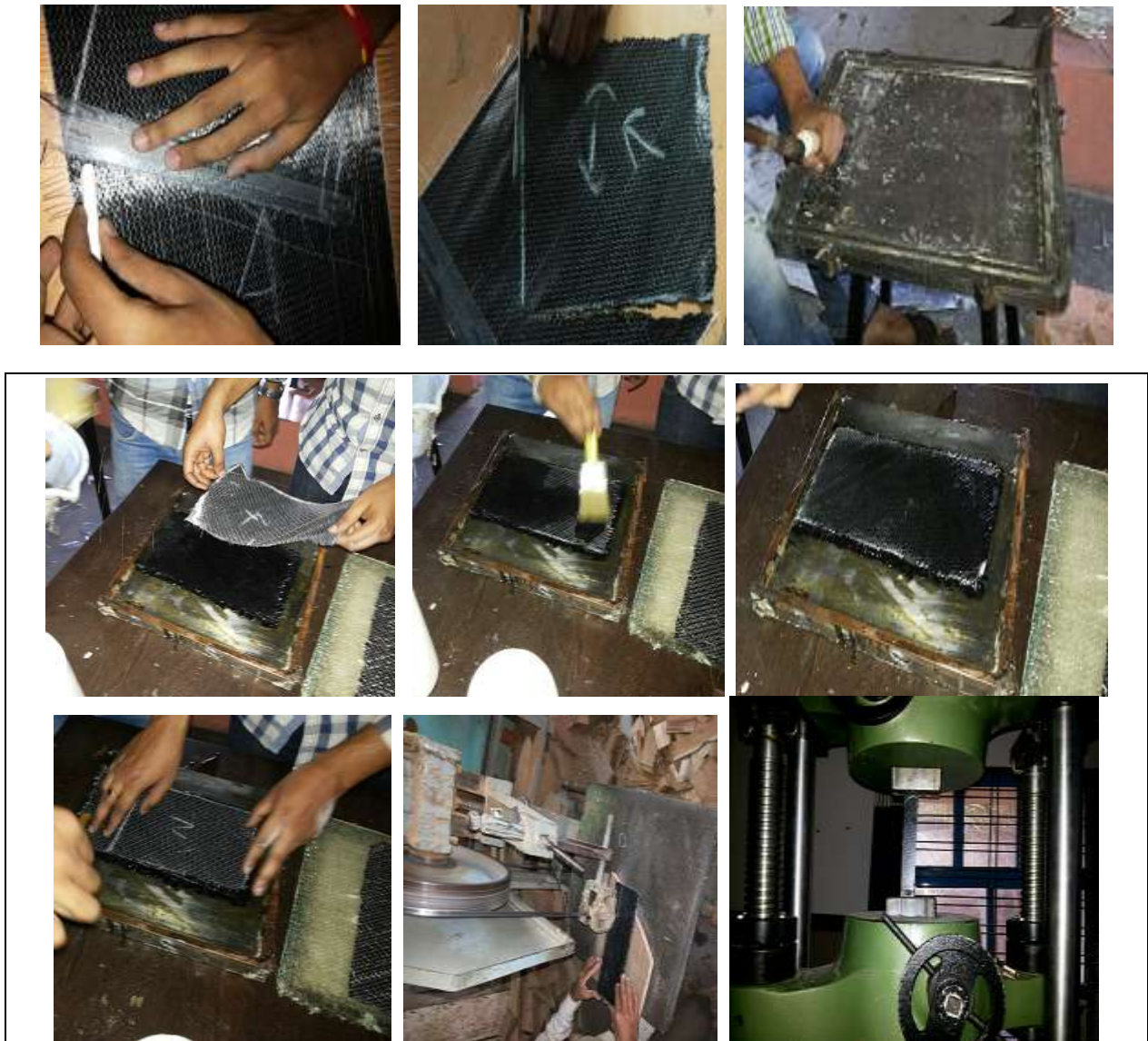
Fig.No.1. various steps for preparation of composite laminate and UTM test
