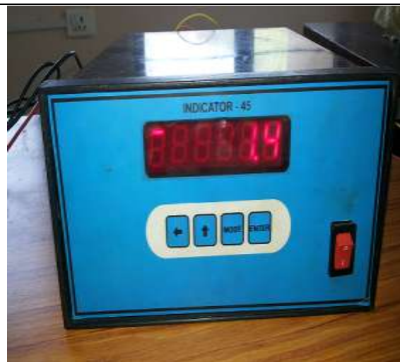
Fig.No.5: Signal Conditioning System
