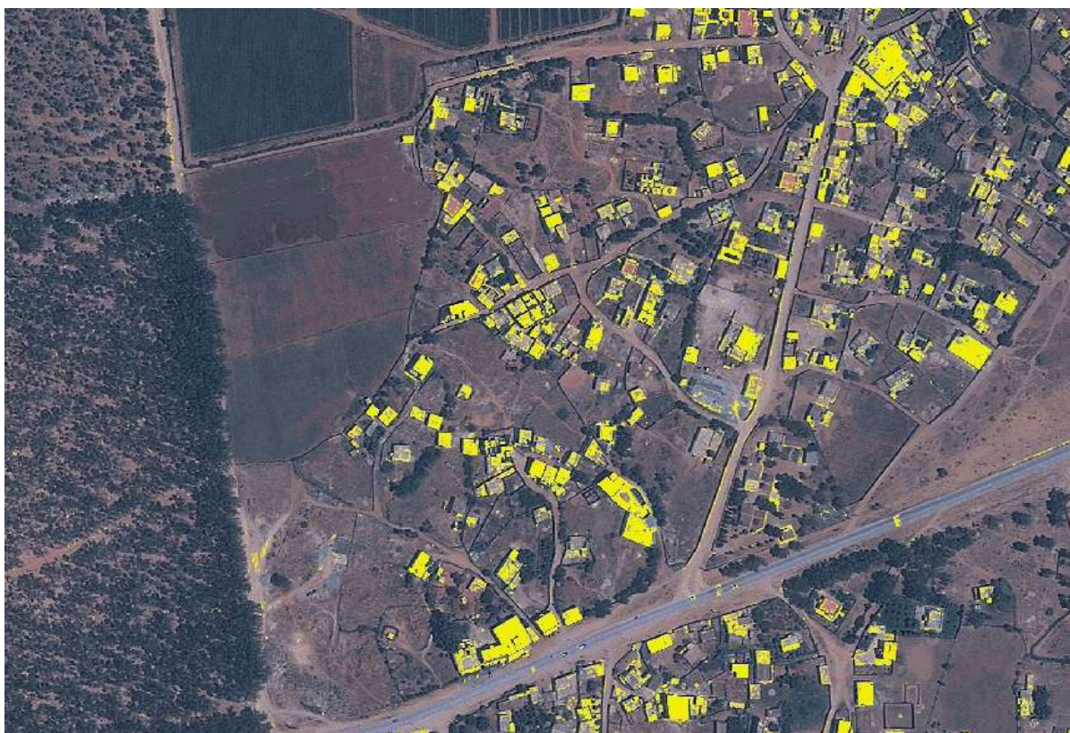
Fig.8: The result of supervised classification using SVM classifier with kernel
