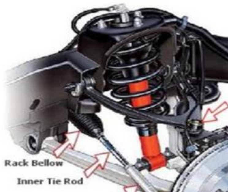
Figure1: Location of tie rod in suspension system
