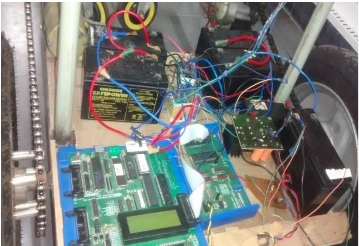
Fig7. Complete wiring connections with batteries, Motors and Wheels of wheelchair
