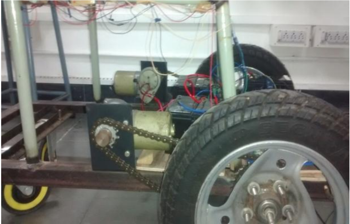
Fig6. Interfacing of motors with wheels
