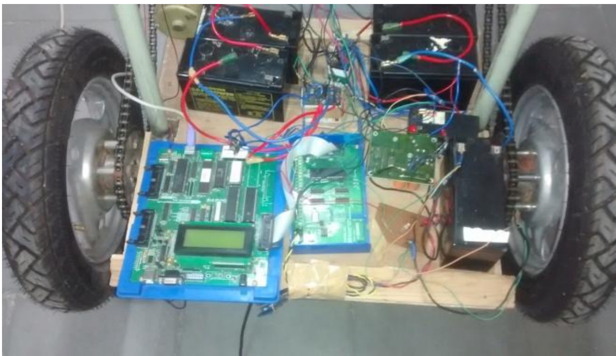
Fig5. Complete wiring of Batteries with board.
