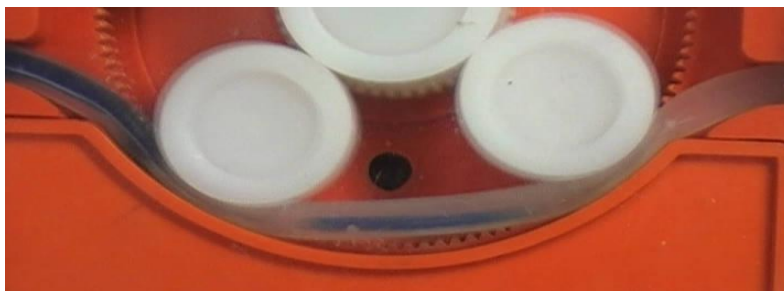
Fig.6: Trapped working fluid in tube between rollers
