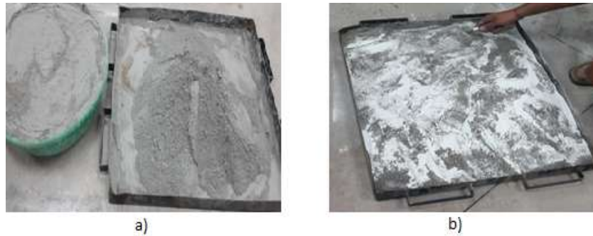
Fig. 4: a) Cement mixed with GGBFS and MWP used in this study & b) Marble Waste Powder mixed with cement
