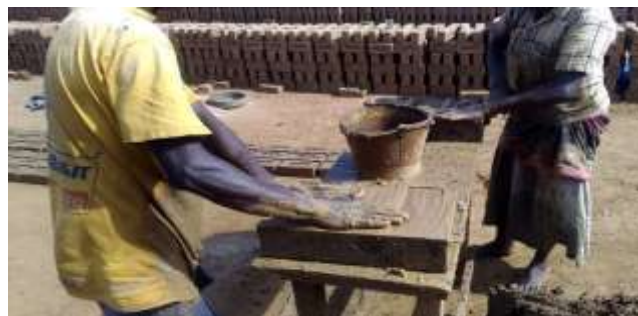
Fig: 6.2 Surface finishing process done by hand.
