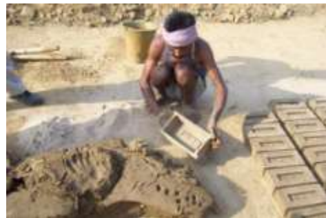
Fig: 3.2 Conventional moulding process
