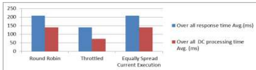
Figure 6: Comparison between Average response time and Dc processing time for three load-balancing Algorithms with the Optimize response time service broker policy
