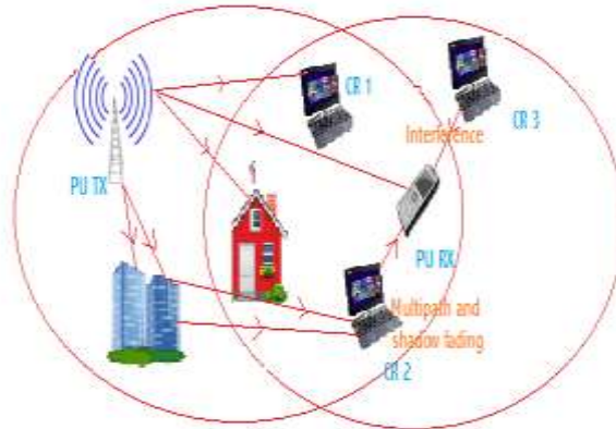
Figure 2: Receiver uncertainty and multipath/shadow fading
