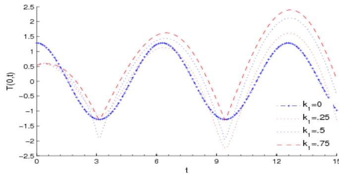
**Figure 2:** Temperature responses with time for the case 2 with different values of variable conductivity  $k_1$
