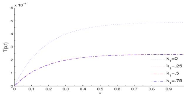
**Figure 4:** Temperature responses with dimensionless distance for the case 1 with different values of variable conductivity  $k_1$
