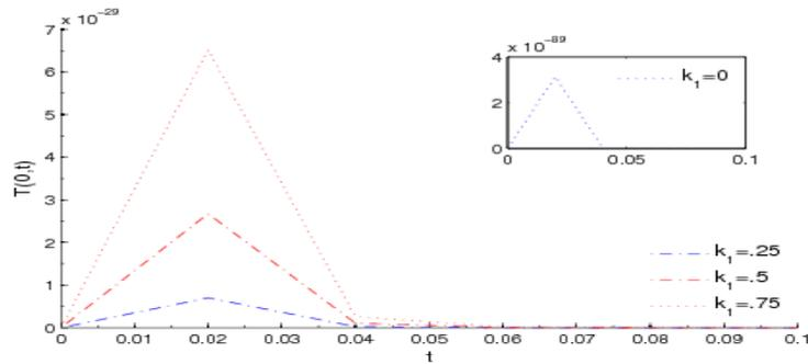
**Figure 1:** Temperature responses with time for the case 1 with different values of variable conductivity  $k_1$
