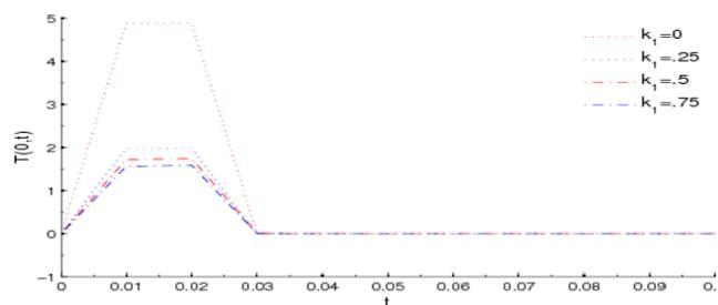
**Figure 3:** Temperature responses with time for the case 3 with different values of variable conductivity  $k_1$
