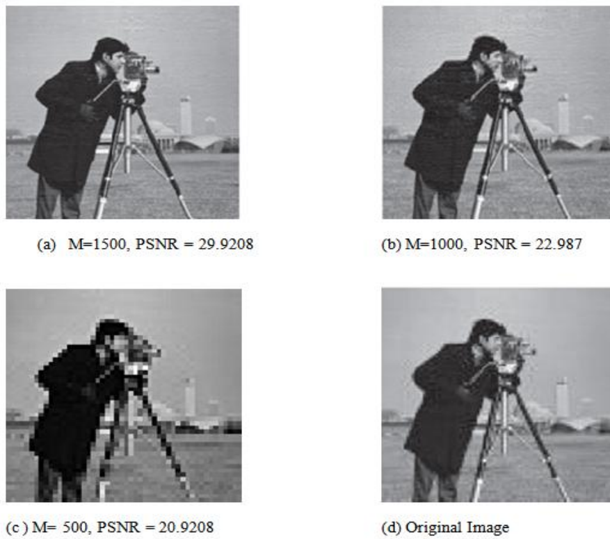
Fig 2: Recovery of Cameraman by Compressive Sensing
