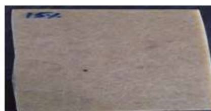
Fig.3.8 Specimen with 20% Microsilica
