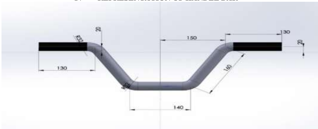
Fig. 4: The handlebar which is introduced in the vehicle to ensure safe and easy handling of the vehicle.
