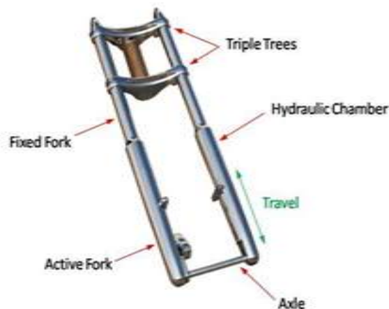
Fig. 2: conventional Tube Fork
