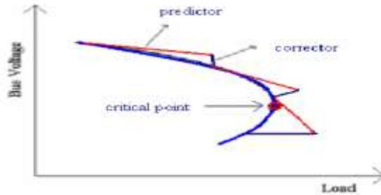
**Fig 1: Bus voltage versus Load**
