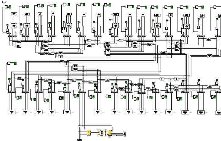
Fig 12: Simulation model of IEEE 30-bus system
