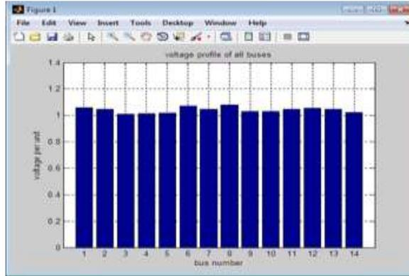
Fig 6: The voltage profile of all buses of the IEEE14 system as obtained from the load flow
