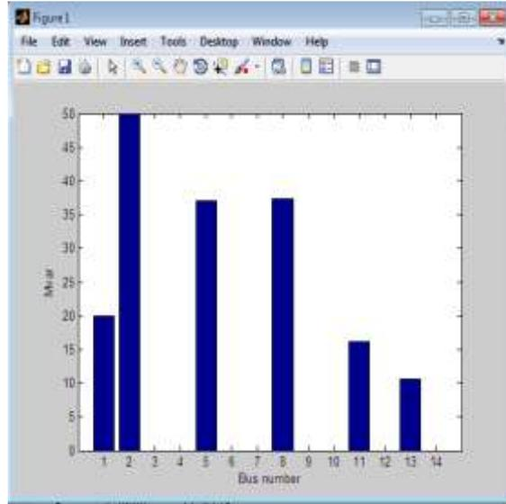
Fig 8: Margin of reactive power in IEEE 14 bus bar test system
