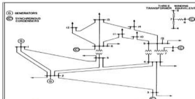
**Fig 2: Single Line diagram of IEEE 14 Bus system**
