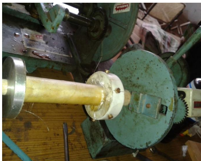
Fig 4: Fibre glass cloth being wound on the former attached to the winding machine
