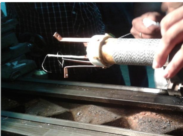
Fig 9 Racquet thread being wound on top of the fibre glass cloth wrapping for reinforcement
