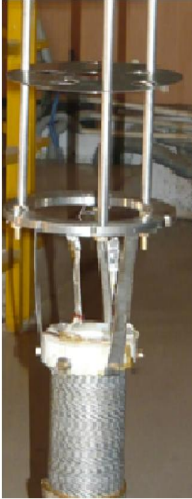
Fig 1: Photograph of lab scale LTS-SC magnet along with support structure to be cooled in a cryostat
