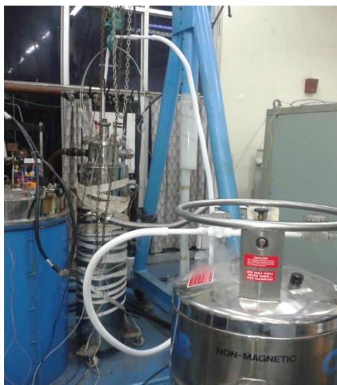
Fig 13: Pre cooling of cryostat using liquid nitrogen
