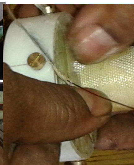
Fig 5 Nb-Ti superconducting wire is being passed through sleeves in a slot on top flange.
