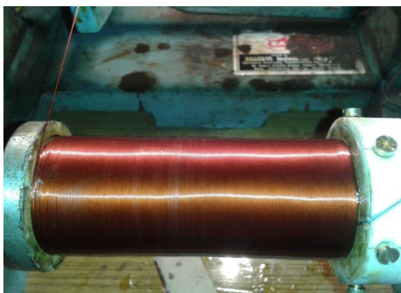
Fig 6 Final layer of superconducting winding, without fibre glass cloth
