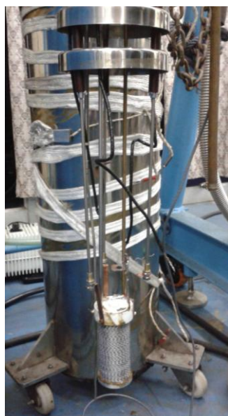
Fig 10: Magnet suspended from top flange by supporting rods shown along with the cryostat for testing.
