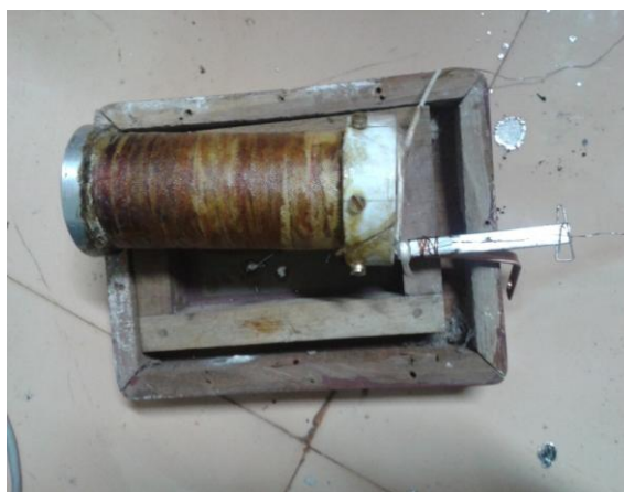
Fig 8 Completed superconducting magnet left for drying of adhesive
