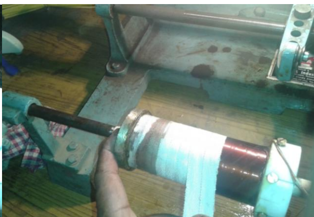
Fig 7 Fibre glass cloth being wound with adhesive on top of the final superconducting coil layer
