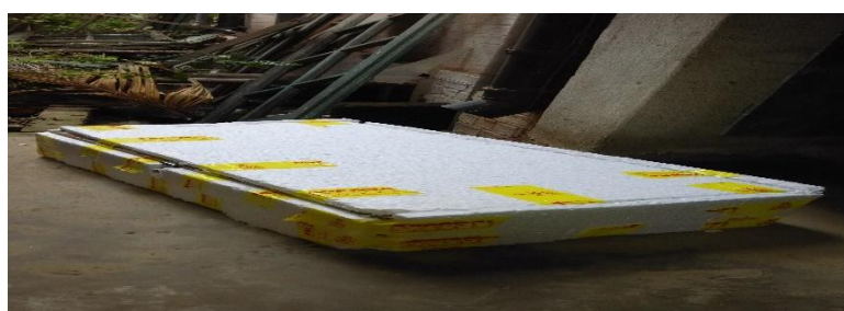
Fig 4: A plywood box covered with thermocoal
