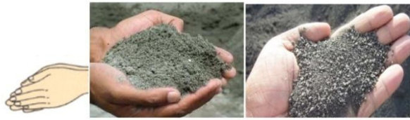
Testing of CS-Sand by “visual observation” and “rubbing with hand” to assess the presence of Quarry dust
