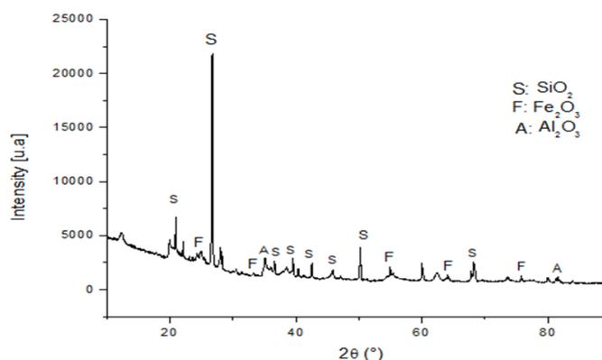
Figure 2 XRD spectrum for  $Fe_2O_3/Kaolin$  catalyst
