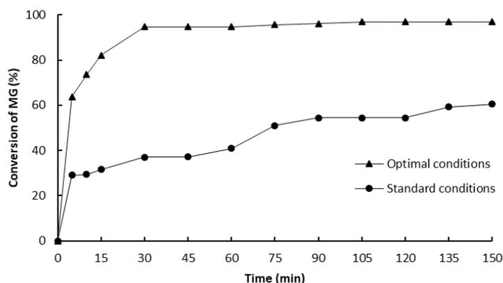
**Figure 9** Evolution of MG conversion along the reaction time under optimal and standard reaction conditions
