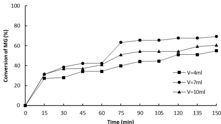
**Figure 7** Effect of  $H_2O_2$  volume on the conversion of MG
