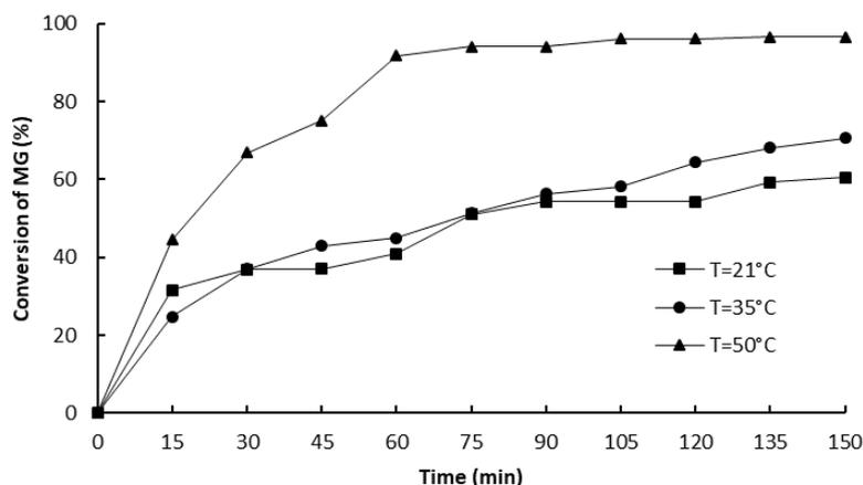
**Figure 5** Effect of processing temperature on the conversion of MG
