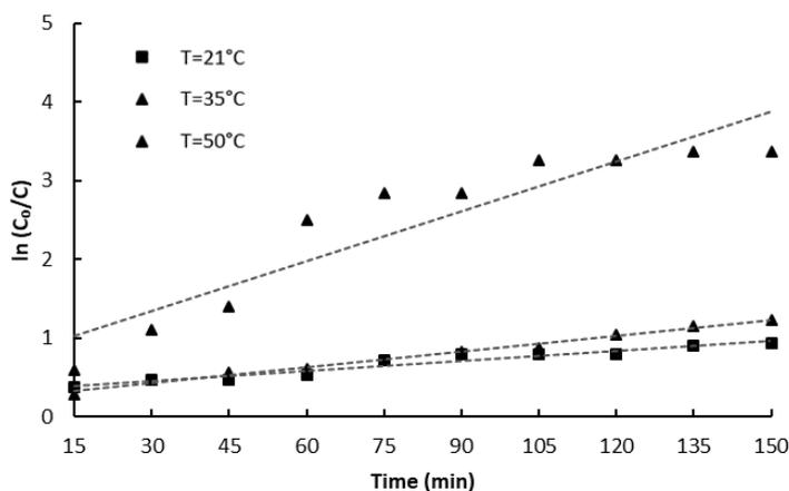
**Figure 6** First-order kinetic plots for WHPCO of MG under different temperatures
