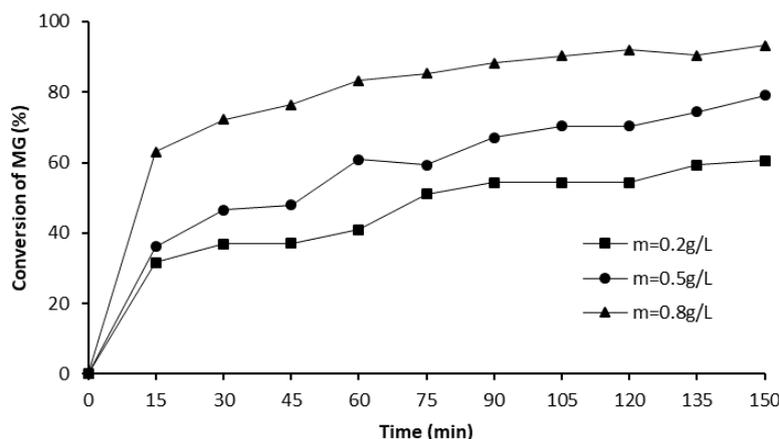
**Figure 3** Effect of catalyst dosage on the conversion of MG
