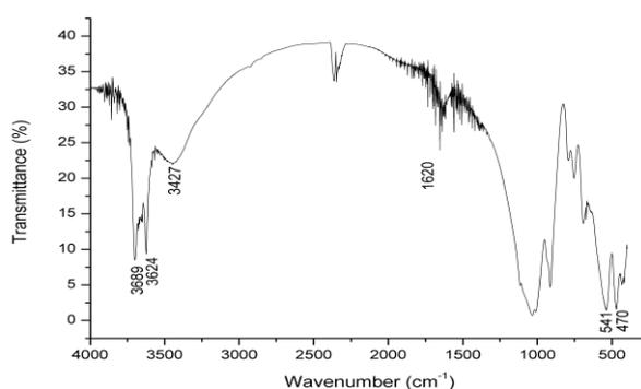
Figure 1 FTIR spectra for  $Fe_2O_3/Kaolin$  catalyst
