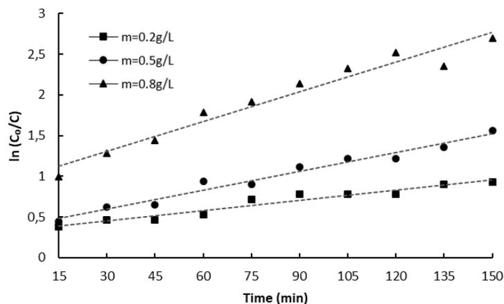
**Figure 4** First-order kinetic plots for WHPCO of MG under different catalyst dosages
