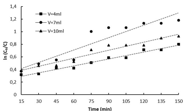
**Figure 8** First-order kinetic plots for WHPCO of MG at different  $H_2O_2$  volumes
