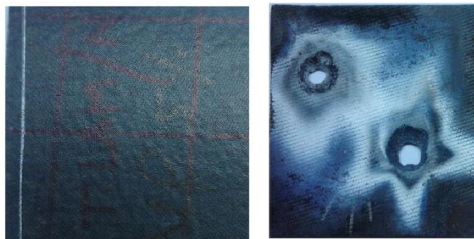
Fig 8, 9 Specimens before & after oxy-acetylene test 5.3.
