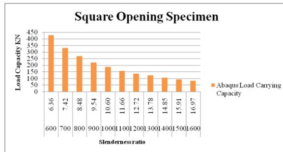
Figure 6 Castellated Steel Column With Square Opening
