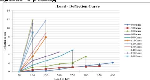
Figure 25 Load Deflection Curve for Tapered Shape with Rectangular Openings
