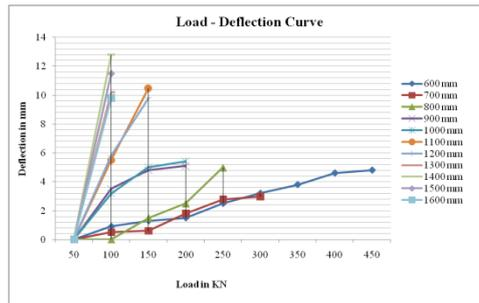
Figure 24 Load Deflection Curve for Tapered Shape with Square Openings
