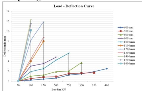
Figure 26 Load Deflection Curve for Tapered Shape with Circular Openings
