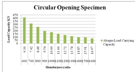
Figure 8 Castellated Steel column With Circular Opening
