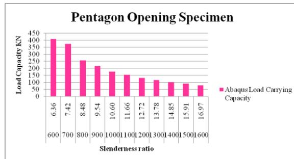
Figure 10 Castelled Steel column With Pentagon opening
