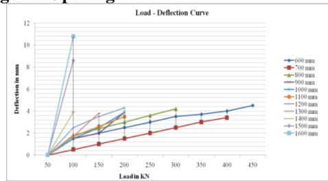
Figure 28 Load Deflection Curve for Tapered Shape with Pentagonal Openings
