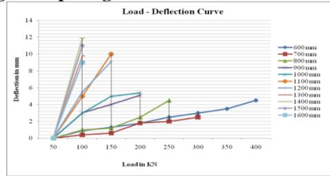
Figure 29 Load Deflection Curve for Tapered Shape with Hexagonal Openings
