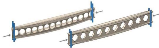
Figure 3 Weak-axis Flexural Buckling Failure Of Cellular And Castellated Members Loaded By A Central Compressive Force
