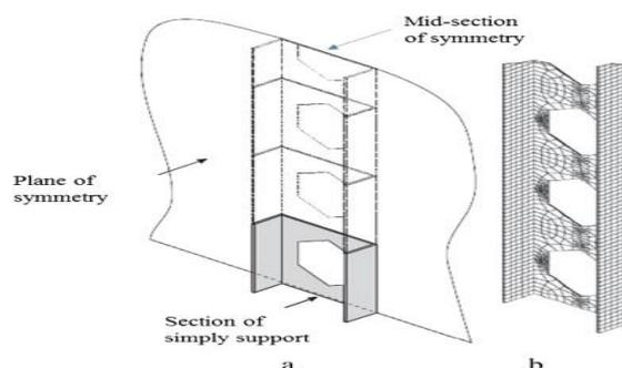
Figure 1 Cross Section of Castellated Column.
