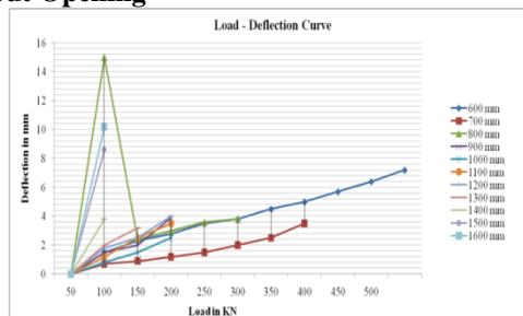
Figure 23 Load Deflection Curve for Tapered Shape without Openings
