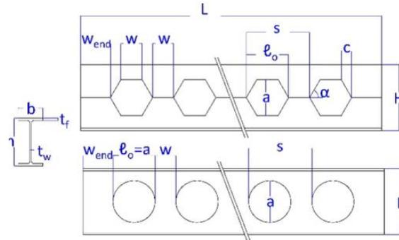
Figure 4 Dimensions Of The Castellated And Cellular Members, As Well As Their Parent Sections
