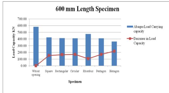
Figure 12 Decrease in Load Capacity of 600 mm Length Of Specimen
