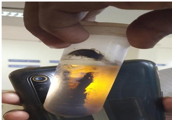
Figure.3. FeNPs attached to the centrifuge tube
