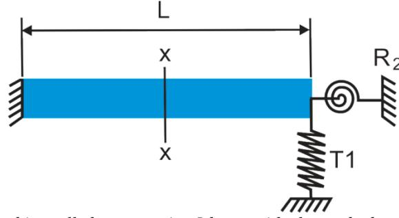
Figure 1 (a). A cantilever thin-walled open section I-beam with clamped edge at one end and Elastically Restrained at the Other End.
