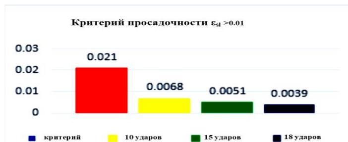
**Figure 4.** Diagram of the average value of the relative subsidence  $\epsilon_{sl} = f(n, W_{opt})$  of compacted soil at different numbers of impacts
