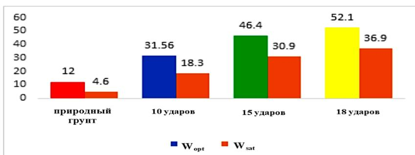
**Figure 5.** Diagram of the average value of adhesion force  $C=f(n, W_i)$  of compacted soil at different numbers of impacts and different humidity
