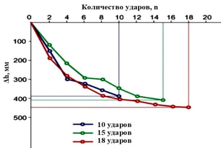
**Figure 3.** Curves of dependence  $\Delta h = f(n)$  for determining the value ( $\Delta h$ ) from the number of blows (10, 15 and 18)
