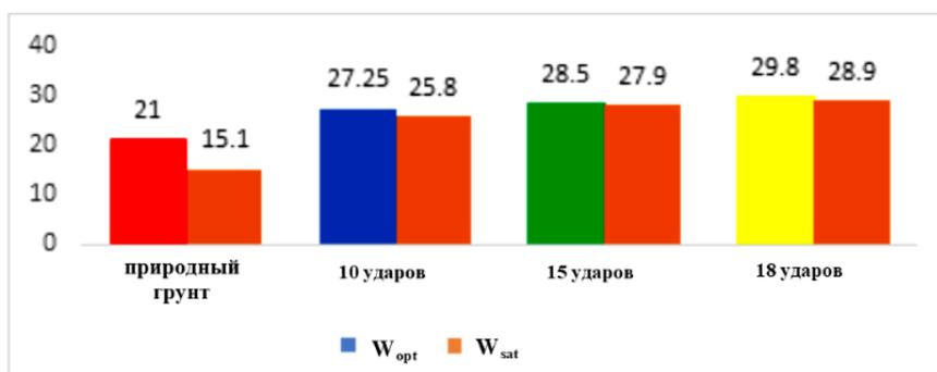
**Figure 6.** Diagram of the average value of the angle of internal friction  $\varphi = f(n, W_i)$  of compacted soil at different numbers of impacts and different humidity
