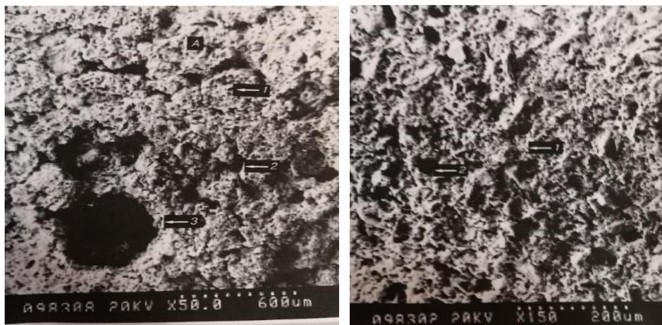
**Figure 1.** Microstructure of loess soil after and before compaction. a - state of the natural structure, c - microaggregate after compaction (x600). 1-micro-unit; 2-micropores; 3-macropores (Sokolov, 1996).
