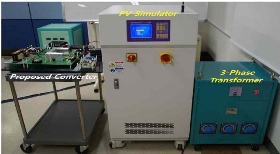
Fig. 12. Experimental setup using the Solarsim-10k PV simulator.
