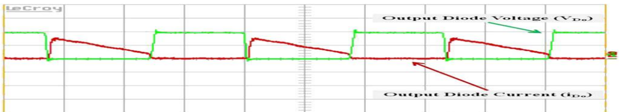
Fig. 16. Measured waveforms of the output diode voltage and current (y-axis: V_{Do} = 200 V/div and i_{Do} = 4 A/div; x-axis: 10 \mu s/div).
