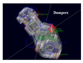
To simulate the actual running of single cylinder engine, the real condition is simulated by mounting the engine of the engine mounting. The engine assembly is mounted on the vehicle mounts with dampers. The vibration coming on the engine at different locations are measured.
