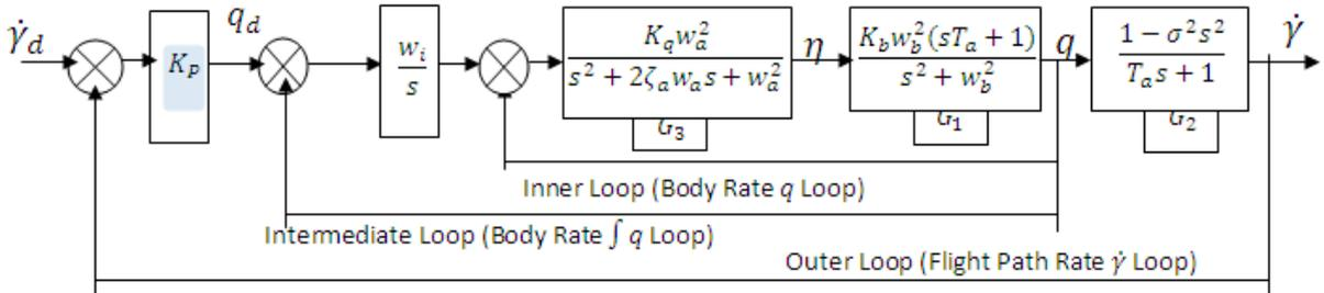
Fig – 2.2: Conventional Three Loop Autopilot Configuration (Transfer Function Model)
