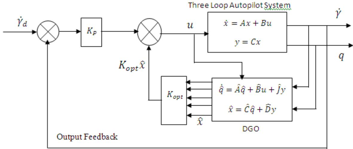
Fig – 2.3: Modified Three Loop Autopilot Configuration using Output Feedback, Das & Ghosal Observer (DGO) and LQR
