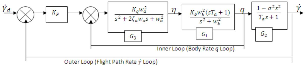
Fig-2.1: Conventional Flight Path Rate Demand Two Loop Autopilot Configuration (Transfer Function Model)
