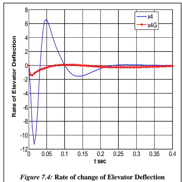
**N.B:** In all of the above four graphs the **blue** lines indicate the classical three-loop autopilot response for frequency domain design approach (as per fig. 2.2) and corresponding state feedback design approach using Ackermann's pole-placement. While the **red** lines indicate the response for LQR based state feedback design methodology along with reduced order Das & Ghosal observer (fig. 2.3).
