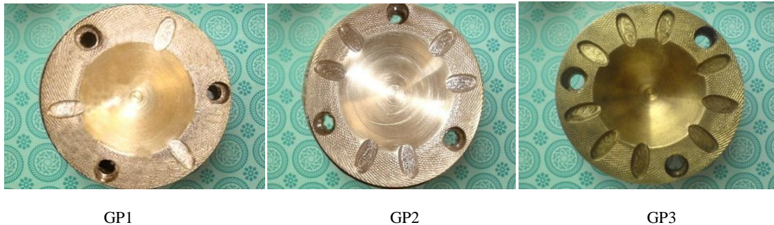
Fig.1 Different types of configurations of piston crowns
