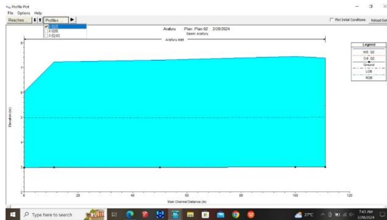
Figure 4: Longitudinal section of the simulation results of the inlet flow to the Arafuru II Retention Pond with a 2-year flood return period (Q 2 )
