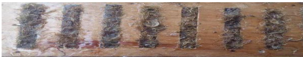
Figure 3.3 Test Specimen Production using the manual Contacting (Open) Molding hand lay up Process
