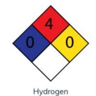
Figure 1: Risk diagram for hydrogen
