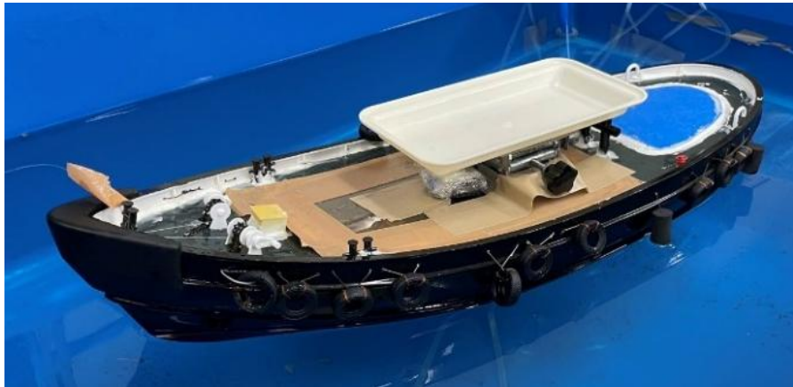
Figure 4 Ship scale model and motion sensor position
