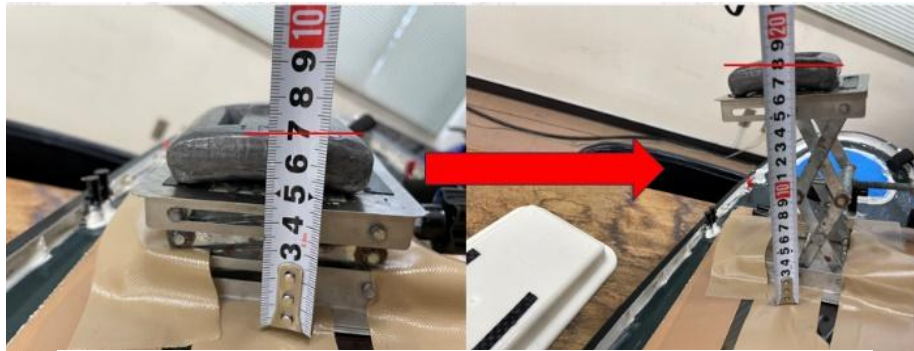
Figure 6 Lifting the shelf from 0.07 m to 0.18 m by 0.01 m increments
