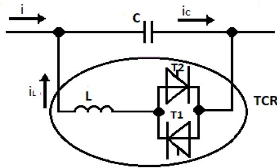
Fig 1. TCSC Controller (Meghwal and Mubeen, 2015).
