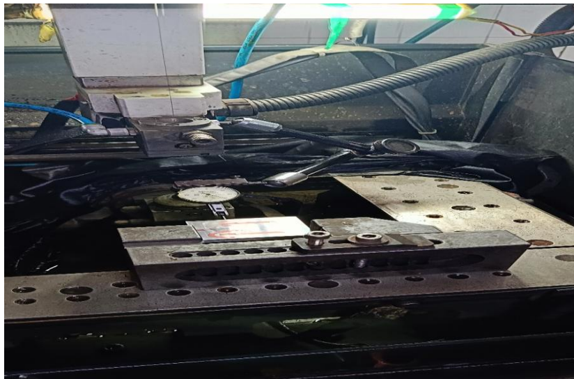
Figure 1: Setup of work piece on WEDM machine.
