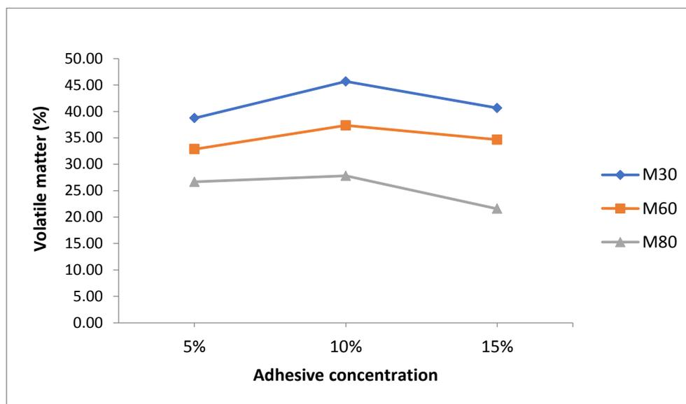
**Figure 3. The relationship of adhesive concentration and particle size on the volatile matter of bio-charcoal briquettes**
