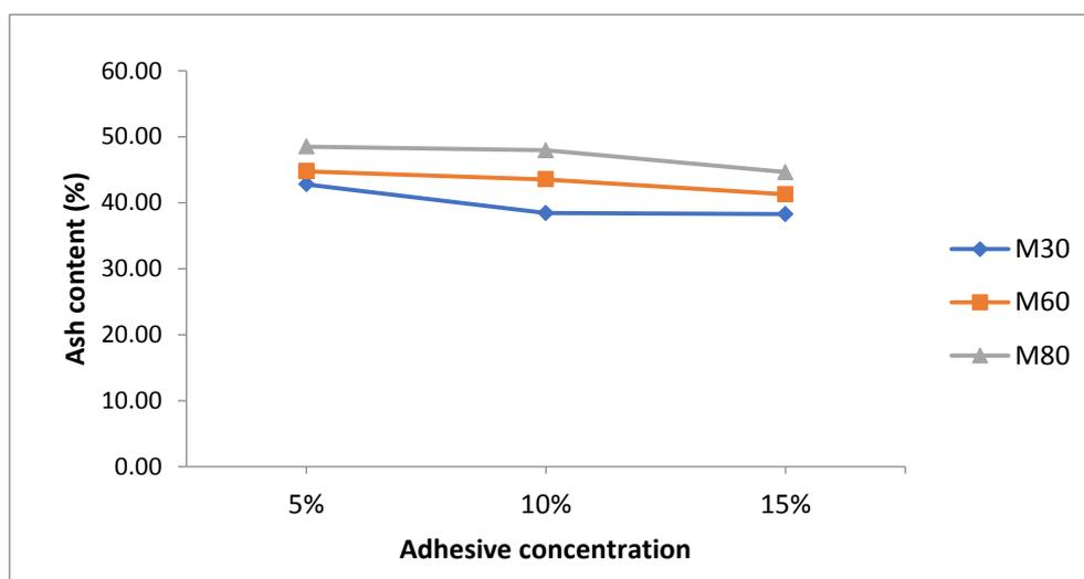
**Figure 4. Relationship of particle size and adhesive concentration on ash content in bio-charcoal briquettes**
