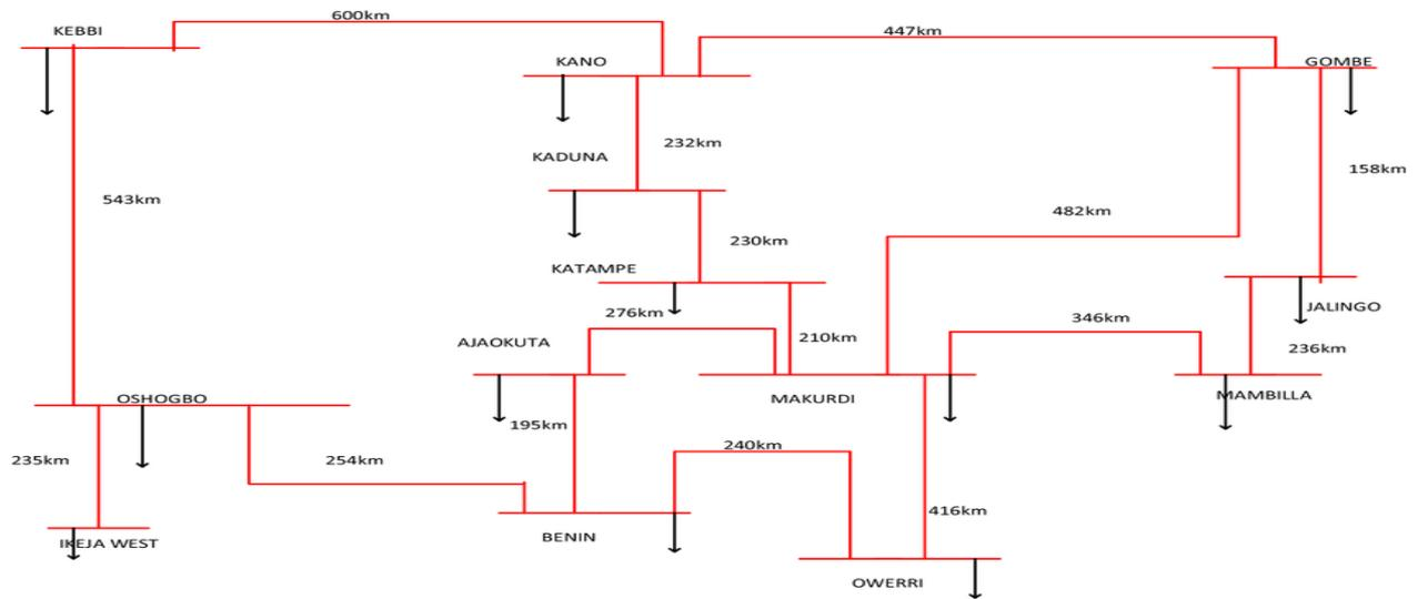
Figure 3: Single Line Diagram of the Proposed Upgraded 750kV Nigerian Transmission Grid (Abdulkareem *et al.*, 2021)
