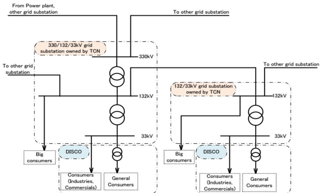
**Figure 1.** Structure of Transmission System (Japan International Cooperation Agency, 2020)
