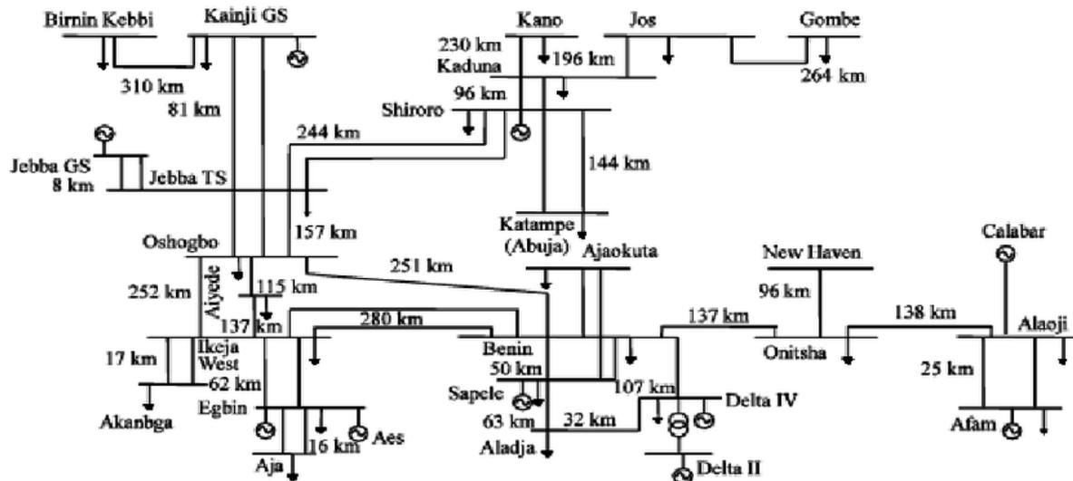
**Figure 2:** One Line Diagram of the Nigeria 330kV Transmission Grid (Okakwu & Ogujor, 2017)
