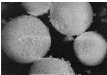
Figure: SEM image of condensed MS (Jaturapitakkul et al., 2004)
