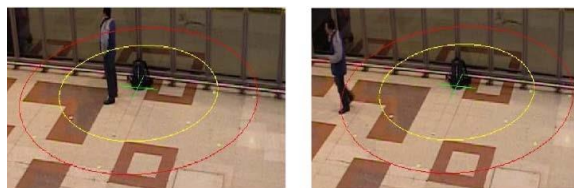
Fig.6. left- distance between bag & person is 2 m(normal). Right- distance between bag & person is more than 2 m(abandoned).
